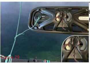
The system are in correct position and the net bag are open, when the ropes are as shown on figure 29.
