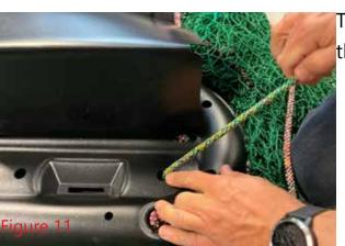
Tighthen the rope so that the plate is tight to the metal pole and secure with a knot.
