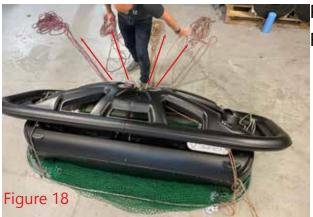
Pull all ropes towards you before placing the Re-Capturing solution on to SeaNest.
