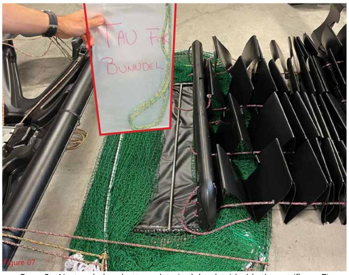
Open SeaNest and place buttom plate (weight plate) inside the net (figure 7)
