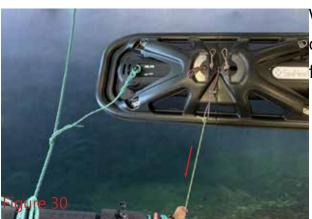
When it it time to catch the cleaner fish, the operator pulls the Pull-Up rope as shown on figure 30.
