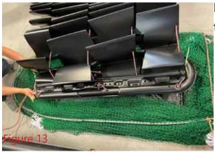
Repeate the connection of the buttom plate to the metal pole also on the other end.
