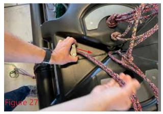
Pull back the rope before launching the system. To be done each time, before launching.
