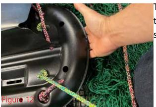
Tighthen the rope so that the plate is tight to the metal pole and secure with a knot as shown on figure.
