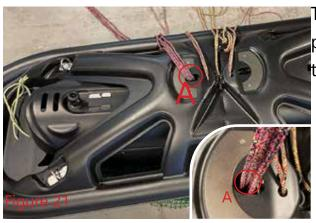
Top part of Re-Capuring solution are in correct position when the 4 ropes from SeaNest are in the centre of hole A.
